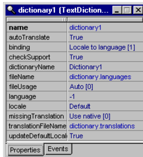
Figure 12. The Properties window showing the properties of a binary dictionary component.
