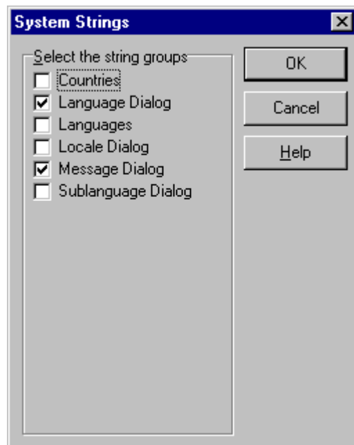
Figure 16. The System Strings dialog box lets the developer add strings used by the system or by the standard components.
